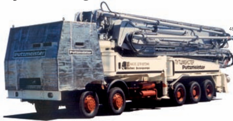
Firstly, truck-mounted concrete pumps were equipped with a lead hood and video control
